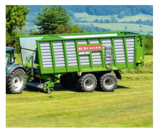
CAREX series loader wagons are available in four tandem models with a DIN load capacity of 37.5 to 43 m³. The hydraulic chassis is standard in all models. They come standard with a movable front wall and a headwall top flap. The scraper floor is made of robust steel and lower at the front for better crop flow and lower power consumption. The 2,050 mm wide pick-up facilitates clean crop pick-up. The theoretical cutting length is 35 mm.
